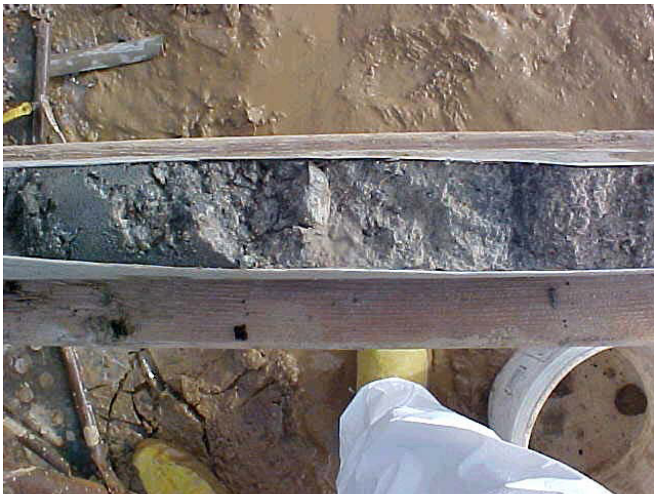
Figure 48. Boring WPZ-11S from 28-30 ft. bgs, showing the presence of gravel ( Weston Solutions 2006 ).
