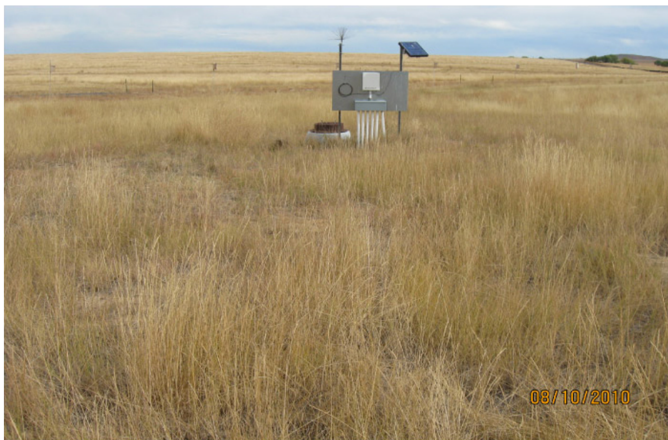
Figure 27. XXX Oil Co.: Trenches RCRA-equivalent cover, postremedy, 2010 (CDPHE 2010).
