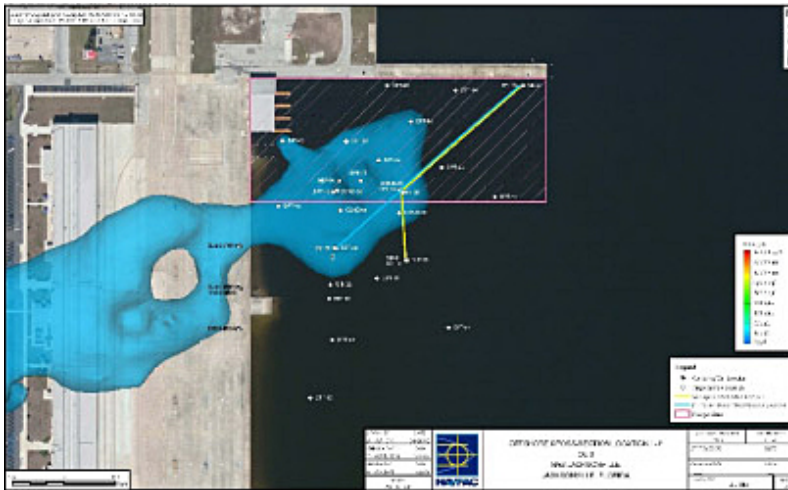
Figure 30. COC plume migrating beneath clay layer in St. Johns River was assessed using trident probe (NAVFAC SE, 2016).
