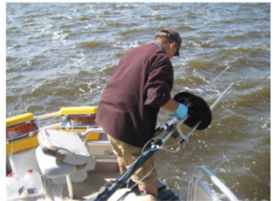
Figure 30. COC plume migrating beneath clay layer in St. Johns River was assessed using trident probe (NAVFAC SE, 2016).
